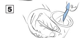
Using a spatula, gently mix the silicone precipitate to blend the different components and evacuate any bubbles.
