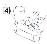
Using a cuter scalpel, remove any stray filaments remaining on the mold. This is finishing stage.
